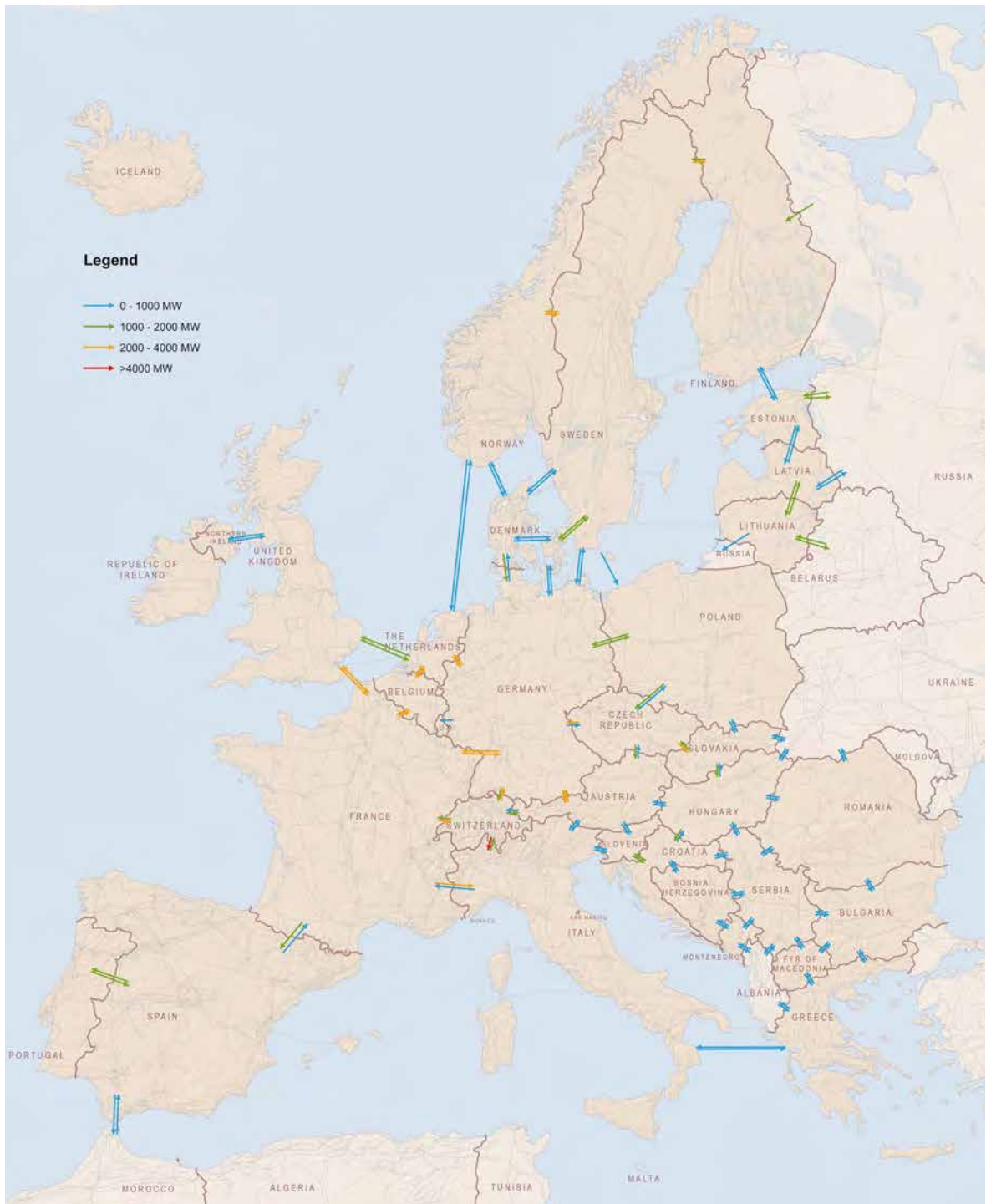
Figure 6.1: Illustration of Net Transfer Capacities in Europe (summer 2010/11)
