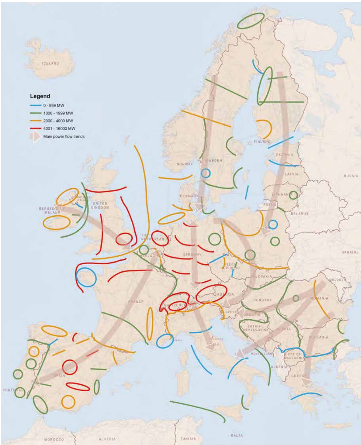
Figure 7.5: Grid Transfer Capability increases
